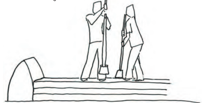
3) Tamp each row and lay barb wire between rows to prevent slipping.
