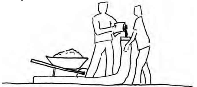
2) Insert can into bag to keep end open. Fill bag with damp soil mixture, and fold end of bag under.
